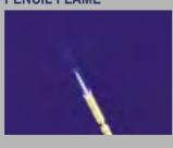
Produces a fine pencil point, which is needed when heat has to be concentrated into a small area. Ideal for detailed and fine jobs.
